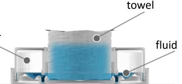
The container (diameter 40mm, height 14mm) is a two-chamber system. In the outer chamber the fluid is held (max 5ml).
