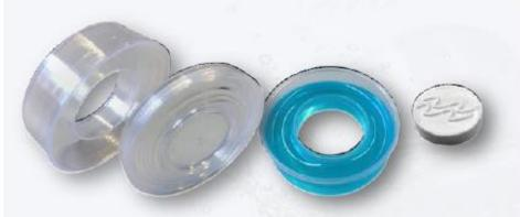
The container (diameter 40mm, height 14mm) is a two-chamber system. In the outer-chamber, the application fluid is held (max.5ml). The inner-chamber holds a compressed cellulose towel (23x22 cm).
